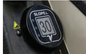
DIGITAL SLOPE INDICATOR Indicates the degree of slope while tractor is in operation.
