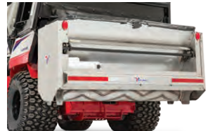
5A250 SIDEWALK DROP SPREADER 2.5 ft 3 /200lbs capacity
