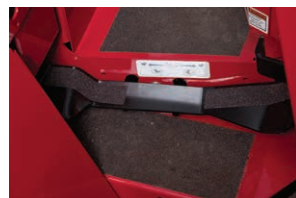
FOOT PEDAL CONTROL A more traditional style foot control for forward and reverse functions.
