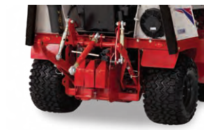
3-POINT Add non-PTO powered implements to the rear with the Category One 3-Point Hitch.
