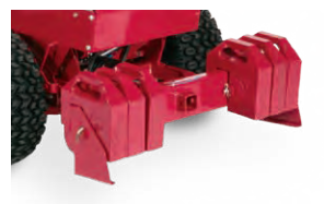
2-N-1 Allows for the option of a front 2-inch receiver hitch or front counterweights.
